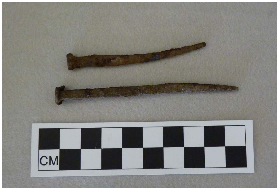
Image 11: (Top) machine cut nail (E115 N111) and (bottom) wrought nail (E115 N111).
