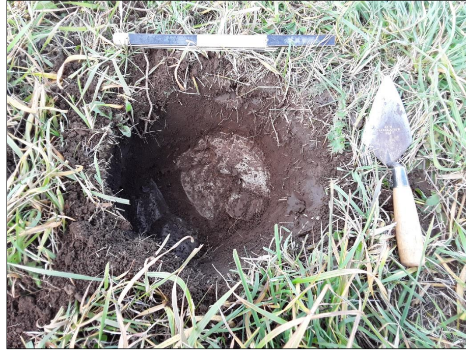
Image 45. Typical test pit showing shallow soil profiles overlying bedrock in north pasture, looking north. (PR20-030D276)
