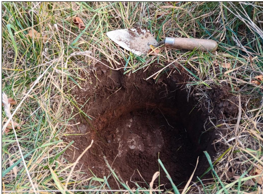
Image 56. Typical test pit showing shallow soil profiles overlying bedrock in fallow land on west side of the study area, looking east. (PR20-030D342)
