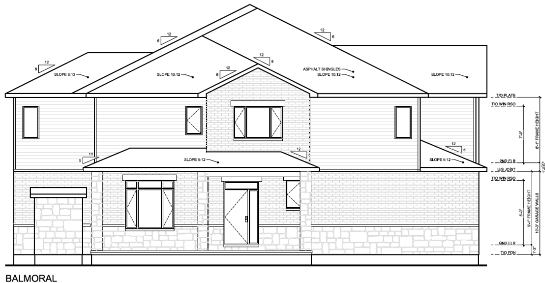
Figure 18: Side building elevation
