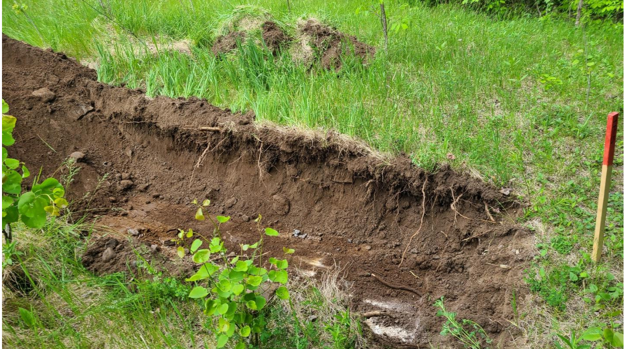
Photo 3: Subsurface profile in Test Pit No. 5
