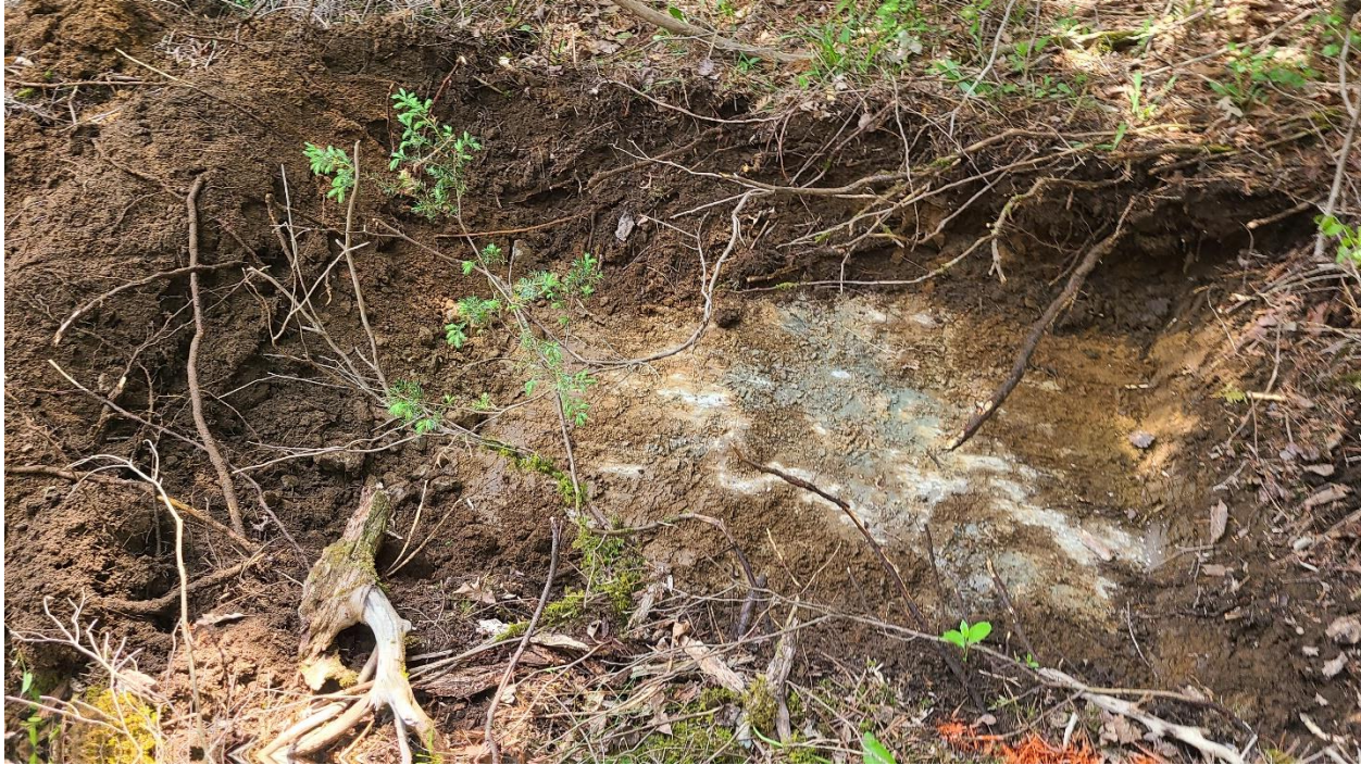
Photo 5: Subsurface Profile in Test Pit No. 11, showing traces of sandy silty clay
